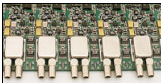
Custom, 7-channel, capacitive position sensor electronics.
